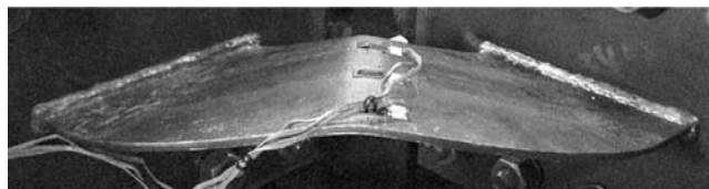
(a) 35-F 圧縮荷時 ( \theta = -0.013\text{rad} )
